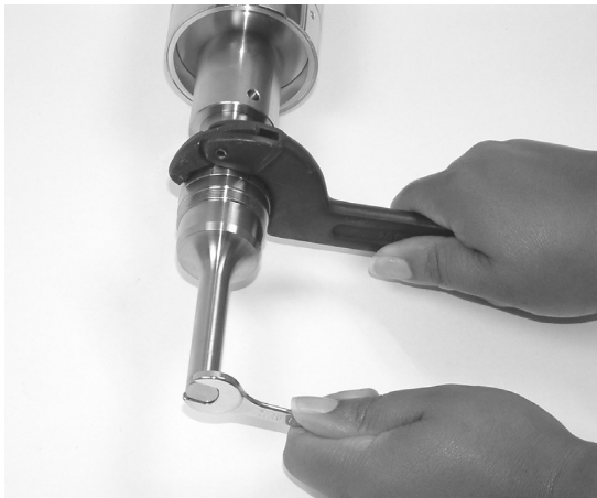
Figure 4.3 Connecting or Removing Tip from Horn
