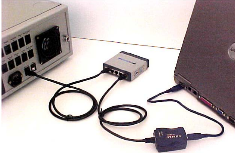
Figure E-13: Connecting one instrument to USB using an Ethernet switch
