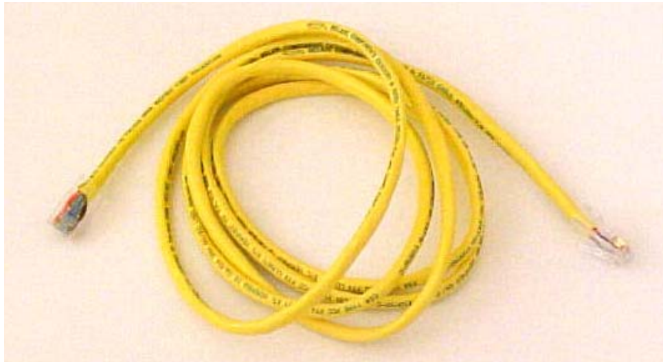
Figure E-4: Ethernet crossover cable shipped by Wyatt Technology
