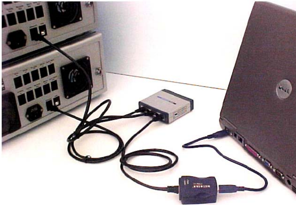
Figure E-14: Connecting two instruments to USB via Ethernet switch and adapter
